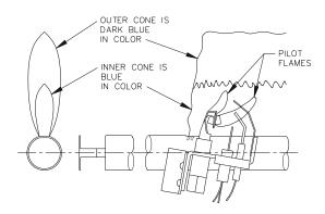
Figure 7: Intermittent Ignition Pilot Configuration and Flames
