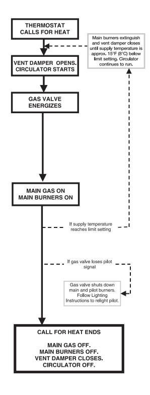
Figure 4: Intermittent Ignition Sequence of Operation
